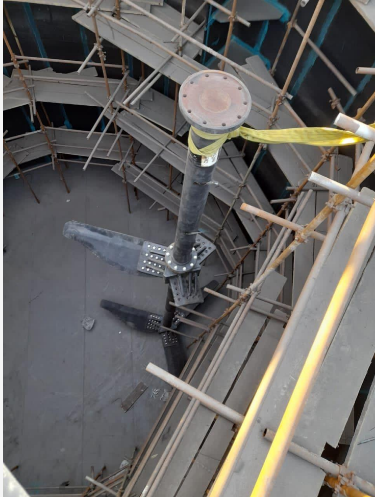
Iron Ore Tailing Agitator, 90kw, 3.7m dia.
