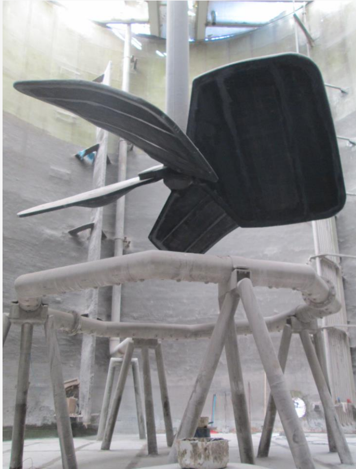
Bioleaching Copper Reactor 110kw, 5.8m dia Weight:18.5 ton
