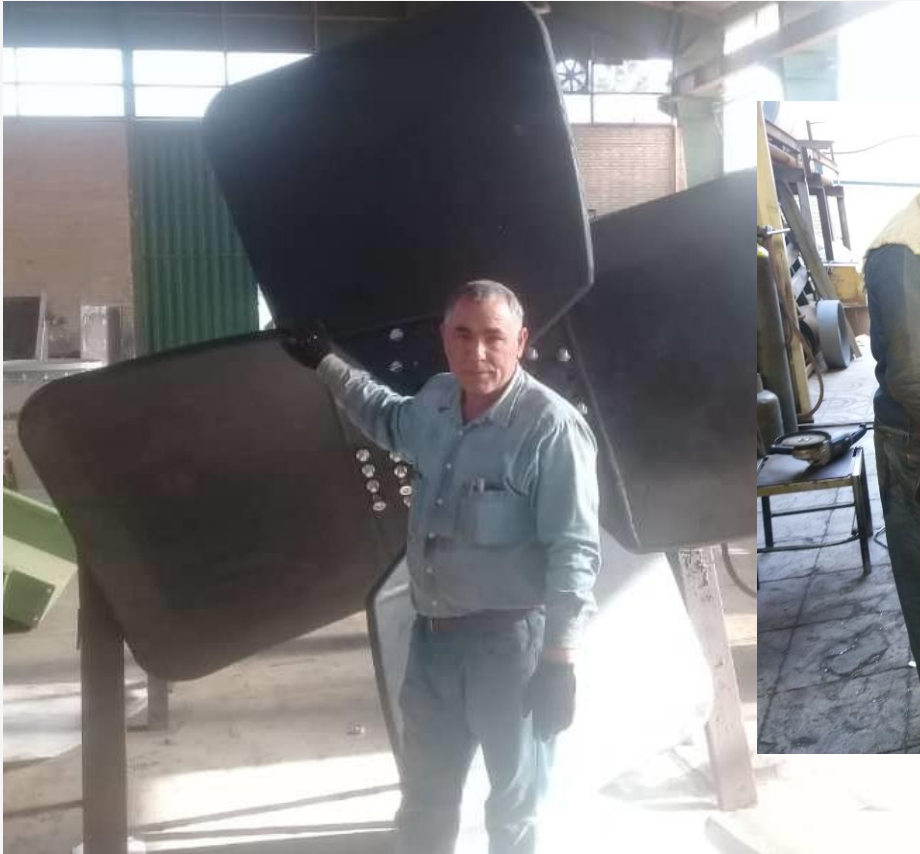
Bioleaching Copper Reactor 22kw, 2.5m dia
