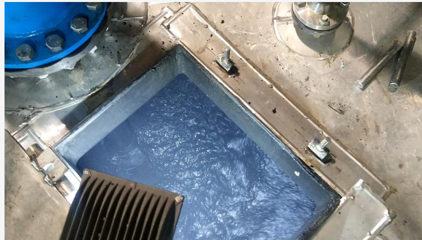
Copper Refinery Stripping Reactor 22kw, 1.8m dia
