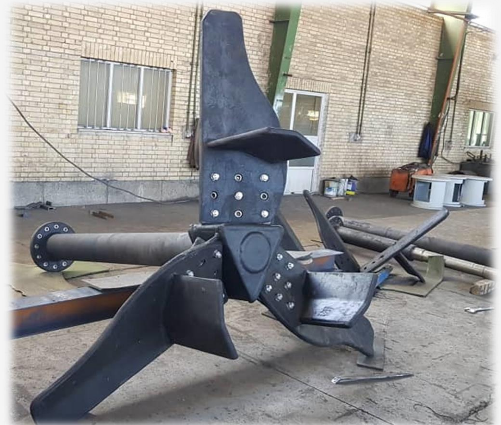
Iron Ore Concentrated Agitator, 55kw, 2.5m dia
